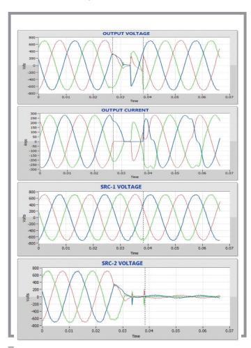
Figure 7: Phase: 120 degree, outage time: 11.50 ms Condition: Loss of source 2
