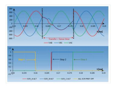
Figure 5: Steps required to transfer the load.
