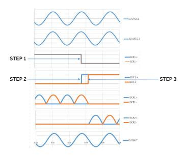
Figure 16: A seamless A9 transfer, synchronized sources
