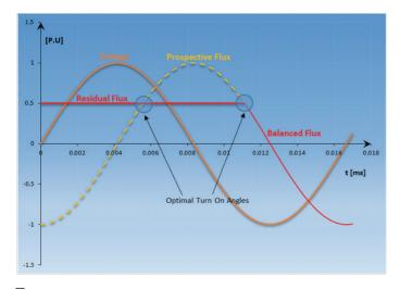
Figure 4: Optimal firing angles
