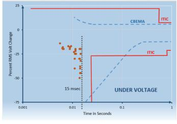
Figure 14: 60Hz data for critical loads meeting CBEMA/ITIC curves.
