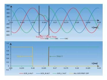
Figure 6: Steps required to do a super transfer
