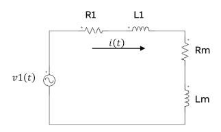
Figure 2: Equivalent Circuit of an unloaded transformer.
