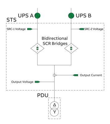
Figure 1: Primary Switching Architecture
