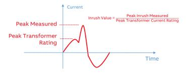
Figure 13: Graphical representation of inrush value
