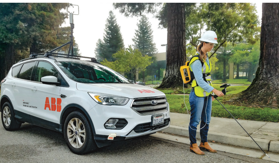
— 01 Tracking leaks with ABB Ability natural gas leak detection solutions: an advanced suite of gas detection systems.
