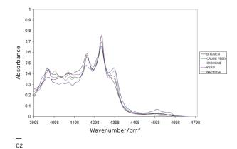
01 Conversion of absorbance spectrum to chemical and physical properties. Calibration models applied to absorbance spectrum to produce values. Calibration models are essentially learning sets with ASTM laboratory reference values.
