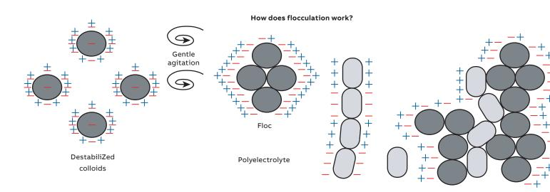
Figure 5 The flocculation process
