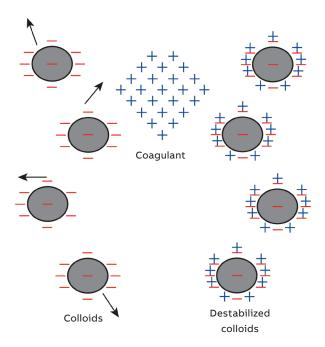
Figure 4 The coagulation process
