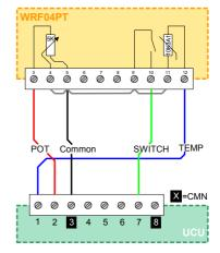
Note: To avoid self-heating, which can affect the accuracy of measurement, the wire current should not exceed 1mA.
