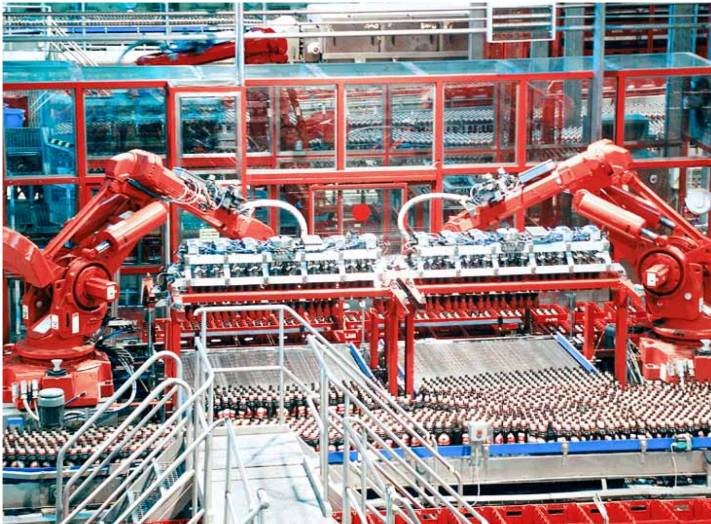
The IRB 6400 robots use a pick-and-place application to identify and remove brand bottles in boxes of mixed returns.
