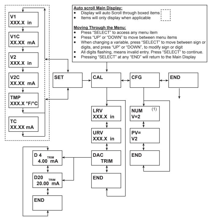
(1) Only displayed when RI100 is NOT in communication with a primary transmitter on power up.
