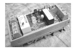
The IFMPGS is mounted on the pillars next to SLOT 2 with the included bolts M3x8. Then the necessary connections are made with the proper wiring, also included.
