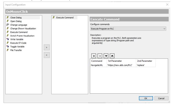
Step 12: Close the Input Configuration, Rebuild the code and download to the processor.
