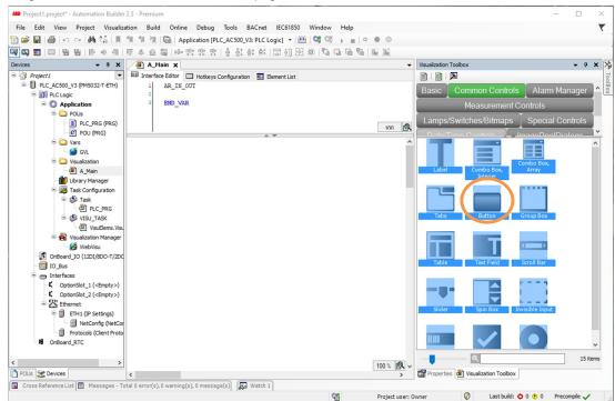
Step 4: With the Button selected, the Button's properties are available in the Properties tab.
