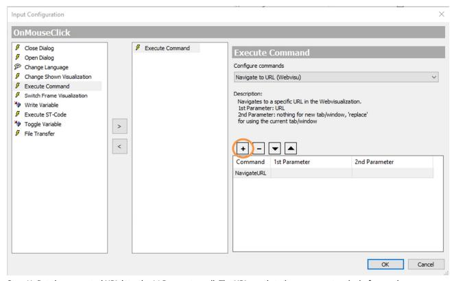
Step 11: Put the requested URL into the  $1^{st}$  Parameter cell. The URL needs to have an apostrophe before and after the full address. Example: 'https://new.abb.com/PLC'
