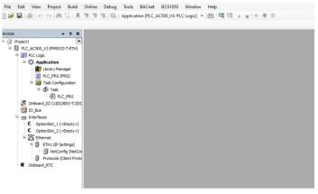
Step 2: Add a Visualization Object and add the Webserver to the Ethernet device in the Interfaces tree
