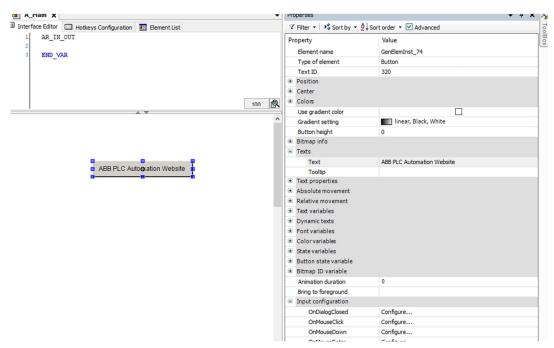
Step 6: Under Input configuration, click on the Configure... text next to OnMouseClick
