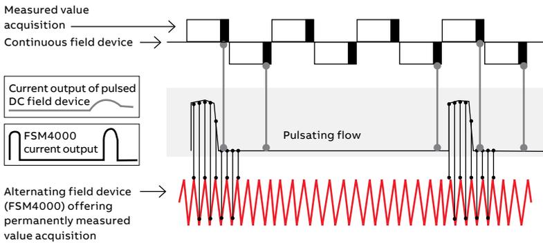
In offering nearly uninterrupted sampling of the flow signal, AC field technology is extremely well suited to measure pulsating flow, generated by piston pumps, diaphragm pumps or hose pumps. Flowmeters working with DC field technology can only acquire pulsating flow data intermittently.
