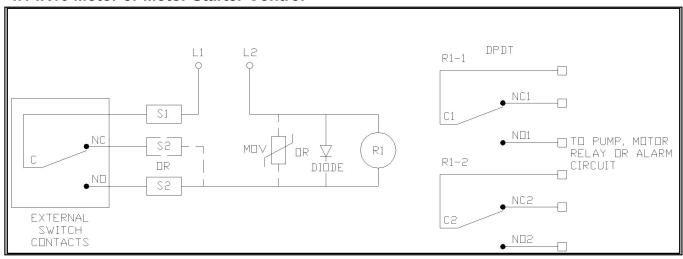
One use of the IR10 is motor and motor starter control. This figure illustrates the proper connection of the IR10 for controlling a motor driven device. Operating power is usually supplied to the IR10 via customer provided AC or DC power distribution panel.
