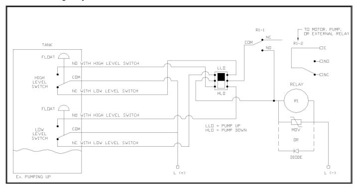
The PP10's primary use is as a latching circuit. This figure illustrates the proper connection of the PP10 for controlling a motor driven device. Operating power is usually supplied to the PP10 via a customer provided AC or DC power distribution panel.
