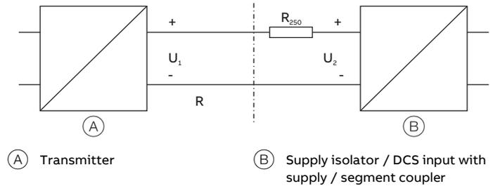
Figure 23: HART load resistance
