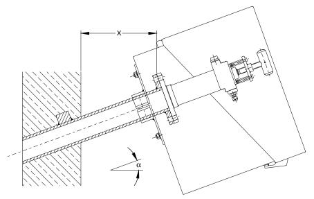
Minimum distance  $x_{min}$  of the mounting flange (wall tube flange) from the wall depending on mounting angle  $\alpha$ :
