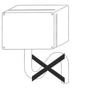
When laying the sample gas line, avoid the formation of water locks, particularly at the sampling points.
