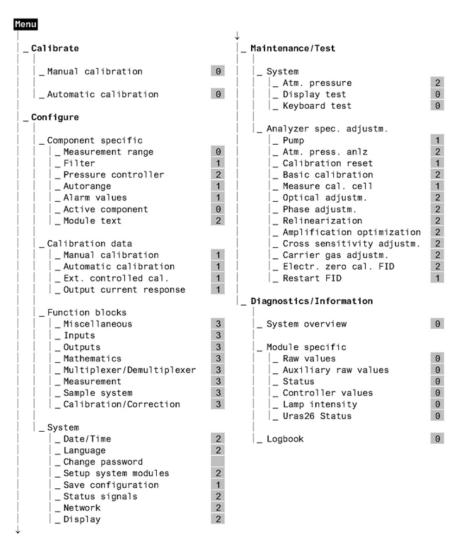
For reasons of brevity only the top-level parameters and functions are shown; the menu branches more extensively at most menu items, e.g. into the various measurement components or into the selection and adjustment of values.
