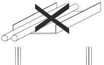
Do not lay the heated sample gas line in a cable tray together with other electrical or pneumatic lines, especially not in an enclosed cable tray.
