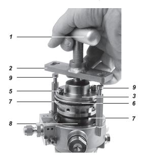
4 Turn detaching disk 3 until it can be pulled off from the hexagon screws 5 via the elongated holes.
