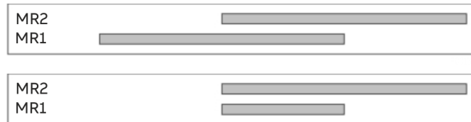
Figure 31: Two measuring ranges with suppressed zero point
