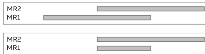
Figure 71: Two measuring ranges with suppressed zero point
