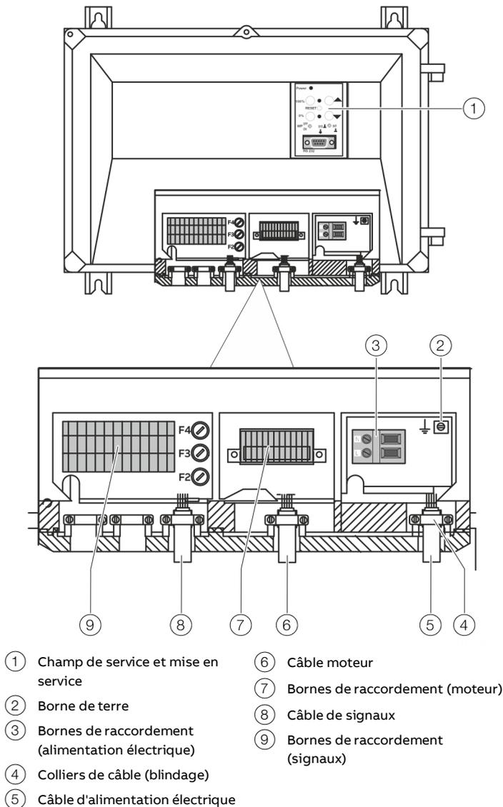
Figure 17 : Zone de raccordement
