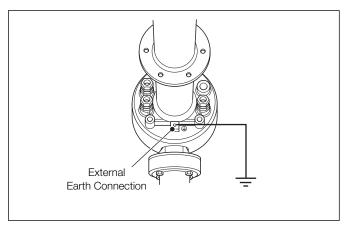
Fig. 5.1 External Earth Connection from Probe
