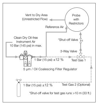
Fig. 4.9 Non-AutoCal with Air as Test Gas 1
