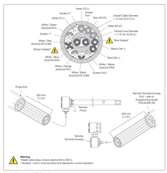
Fig. 5.3 Preparing the (ABB) Probe Cable
