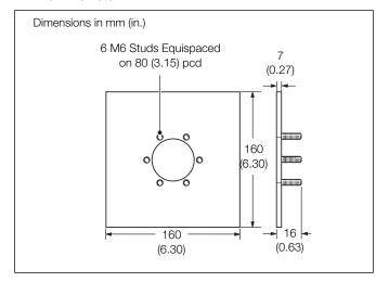
Fig. 4.15 Standard Mounting Plate - 0.5 m (1.7 ft) Probe
