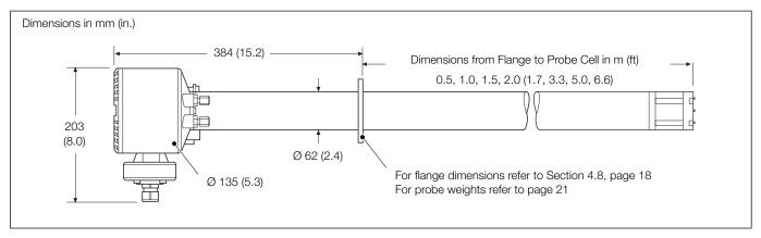
Fig. 4.13 Overall Dimensions – Remote Endura AZ30 Probe
