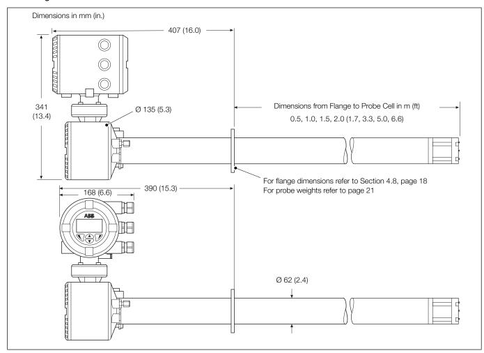
Fig. 4.14 Overall Dimensions – Integral Endura AZ30 Probe
