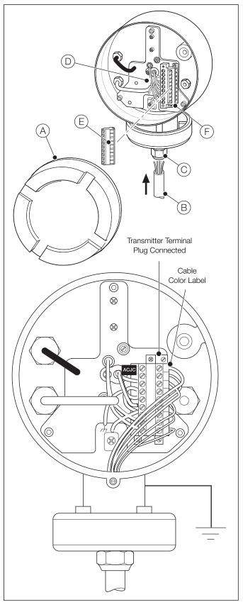
Fig. 5.5 Endura AZ30 Probe Cable Connections
