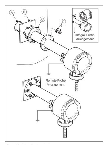
Fig. 4.18 Mounting the Probe
