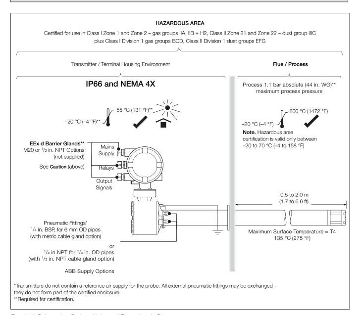
Fig. 4.11 Schematic - Probe with Integral Transmitter In Situ
