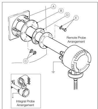
Fig. 4.19 Adaptor Plate Mounting – 0.5 m (1.7 ft) Probe to Large Probe
