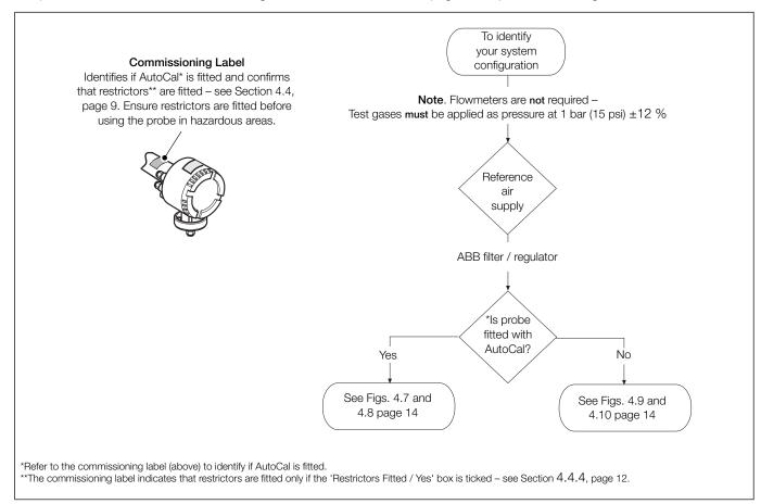
Fig. 4.6 Pneumatic Connection Configurations
