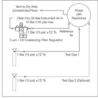
Fig. 4.8 AutoCal with 2 Test Gases
