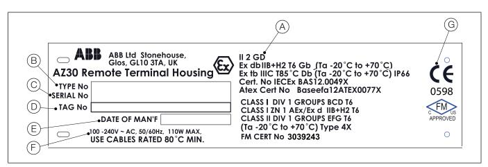
Fig. 4.4 Remote Terminal Housing Label
