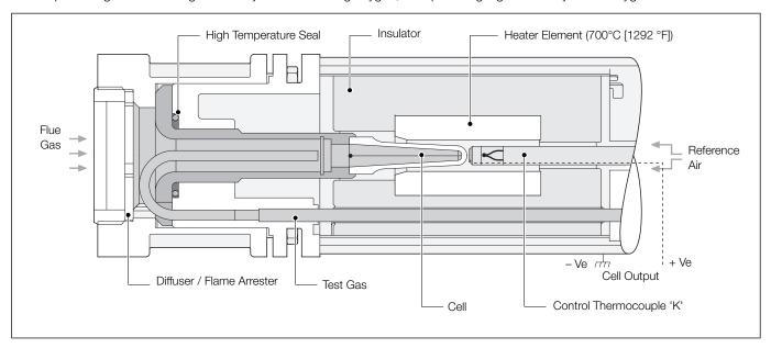
Fig. A.1 Endura AZ30 Probe Construction
