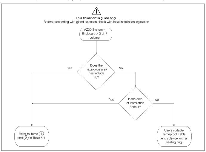
Fig. 5.2 Cable Entry Selection Flowchart
