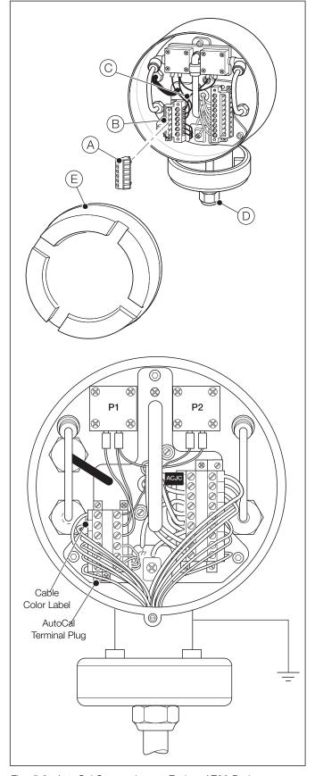
Fig. 5.6 AutoCal Connections at Endura AZ30 Probe
