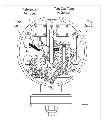
Fig. 5.12 Internal Test Gas and Reference Air Tubes – AutoCal Fitted
