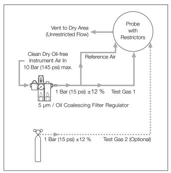
Fig. 4.7 AutoCal with Air as Test Gas 1
