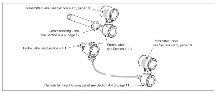
Fig. 4.1 Location of Probe and Commissioning Labels
