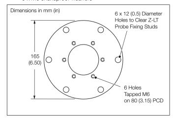
Fig. 4.17 Long Probe to 0.5 m (1.7 ft) Probes Adaptor Plate
