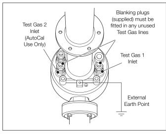
Fig. 5.8 Test Gas Connections – Endura AZ30 Probe with Remote Transmitter Shown
