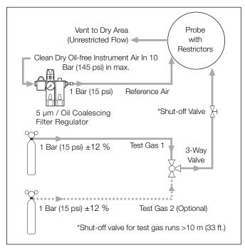
Fig. 4.10 Non-AutoCal with 2 Test Gases
