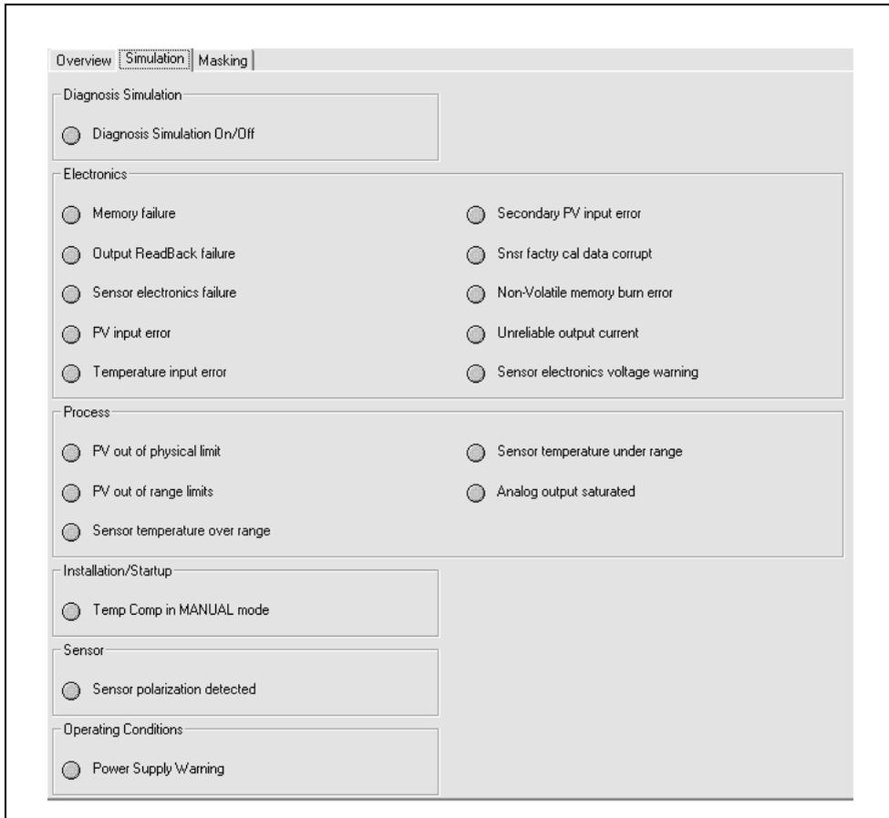
Fig. 8.4 ACA592 2-Electrode Conductivity Transmitter – Diagnosis Simulation Screen
