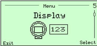
Used to configure and format the information displayed, including: language, data displayed on Operator Pages 3 and 4 and screen contrast.
