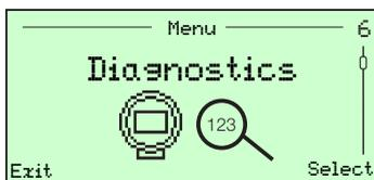
Used to perform a loop test (output verification) and indicate the diagnostic status (actual / simulated).
