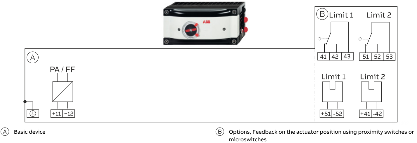
Figure 20: Electrical connection TZIDC-210, TZIDC-220
