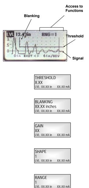
Note: After setting the value of each function, pressing the SELECT button will return you to the WAVEFORM screen.
