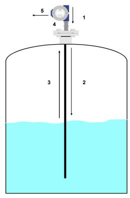
A simplified signal trace as seen on the graphic display (Figure 1) can be divided into three identifiable sections: Coupler Reflection, Signal Reflection and End of Probe Reflection.
