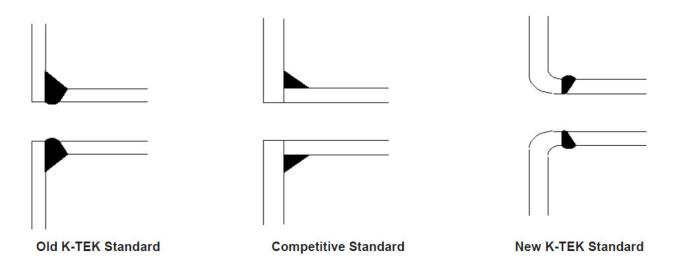
New ABB/K-TEK Standard: Extruded outlet. This outlet is made in three steps. (1) In the first step an ellipse is cut into the pipe. (2) Then a forming head inserts into the pipe. Forming pins retract from the forming head and the head is pulled out of the pipe while spinning. (3) A third operation mills a butt-weld end prep.
