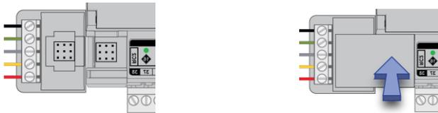
**Note** The termination block can only be used on the **right-hand** interlink connector of the last **FLX** unit on the FLX bus.
