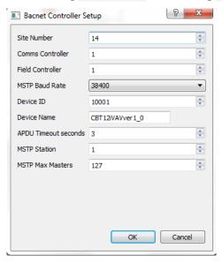
7. From this window the BACnet MS/TP configuration settings can now be configured.
