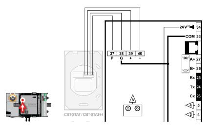
Alternatively, the diagram below illustrates the connection between CBV-2U4-3T(-N) and a typical standard room sensor with a space temperature type III thermistor, including a 5K setpoint slide adjust.
