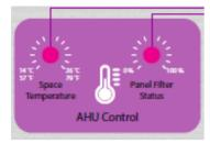
FLX02: UI02 - Drives to Alarm when simulated pressure differential across filter increases. Potentiometer + Uniput 209 (Analog LED). Alarm resets on removal.
