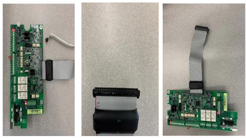
Step 8: Mount the 64652745 (OPEX-01 Interface Board) onto the control board (SMIO-01). The 64738852 – Connection Cable connects to the 8-pin connection on the 64652745 (OPEX-01 Interface Board) and the RJ45 connector of the 64738852 connects to the removed control panel (SMIO-01) through the cutout on the 64652745 (OPEX-01 Interface Board).
