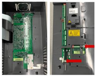
Step 6: On the back plane of the board and plastic housing push the 4 tabs that hold the board in place away from the control board (SMIO-01). Lift board and slide it out of the plastic cover of board enclosure.
