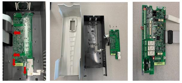
Step 7: Remove small ribbon cable connector from control board (SMIO-01). You keep the existing ribbon cable with 40 pin connector in place.
