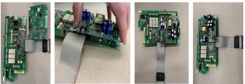
Step 9: Connect your 24VDC power to the 2 terminals on the 64652745 (OPEX-01 Interface Board)
