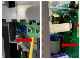
Step 5: After disconnecting the ribbon cables, remove the plastic board enclosure with the control board (SMIO-01) still mounted in it. Remove the mounting screws from the front panel to complete removing the permanent fixtures keeping the board in place in the plastic housing.
