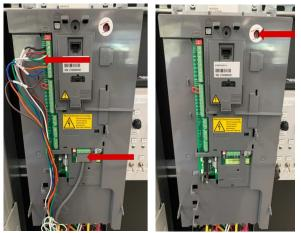
Step 4: At the bottom of the plastic board enclosure there will be two plastic tabs (on bottom left, one bottom right) that should be pulled down to separate the enclosure. After they are pulled down, slowly separate the plastic board enclosure housing about 1 -2 inches to see the two ribbon cables that must be detached from the unit to free the control board (SMIO-01).
