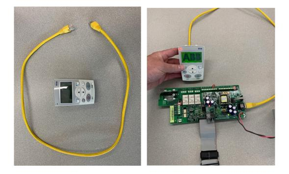
Step 2: Navigate to parameters on the control panel (ACH-CP-B), changed parameters and record all changed parameters.
