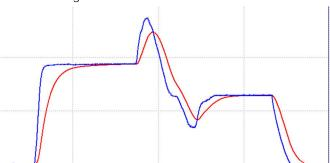
Below is a graph of the encoder speed reference (Blue) compared to the drive speed (Red) after parameter 46.11 was set to zero.
