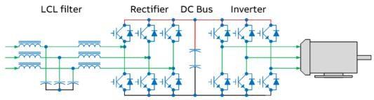
Figure 2 Active front end drive schematic
