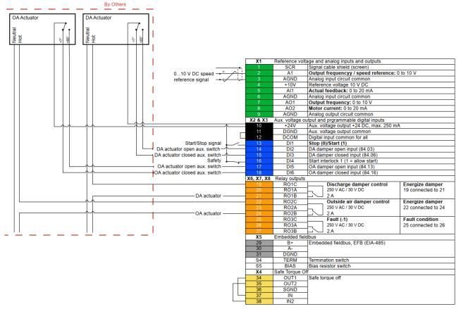
Diagram 2: Outside Air + Discharge Air Damper
