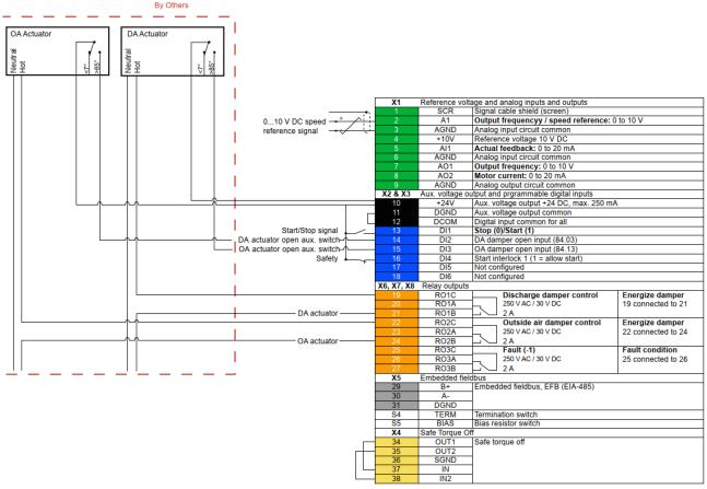
Diagram 3: Outside Air + Discharge Air Damper with only open auxiliary switch
