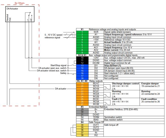
Diagram 1: Discharge Air Damper with or without pre-pressure
