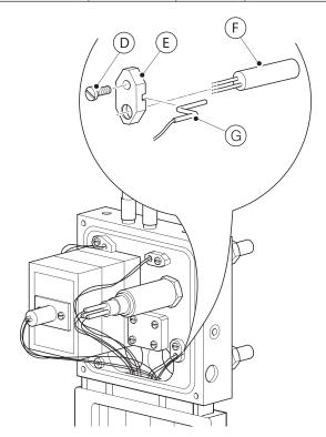
Fig. 8.5 Replacing flange block thermocouple (T/C 2)
