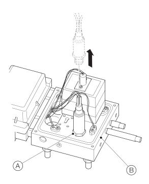
Fig. 8.3 Removing the O<sub>2</sub> sensor
