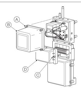
Fig. 7.1 Removing sensor covers
