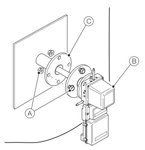
Fig. 5.4 Removing the sensor assembly from the process
