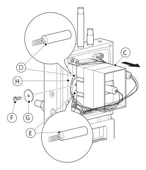
Fig. 8.2 Replacing CO heater block cartridge heaters (70 W)
