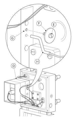
Fig. 8.4 Replacing CO heater block thermocouple (T/C 1)
