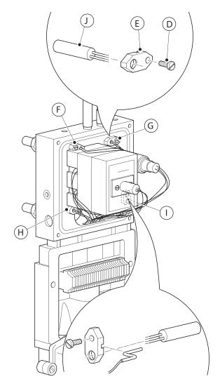
Fig. 8.1 Replacing flange block cartridge heaters (100 W)
