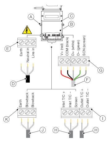
Fig. 5.3 Disconnecting sensor cables
