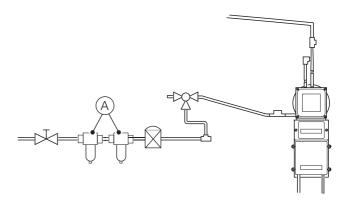
Fig. 8.6 Replacing filter elements in 2-stage filtration system
