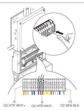
Fig. 8.3 Removing the O2 sensor
