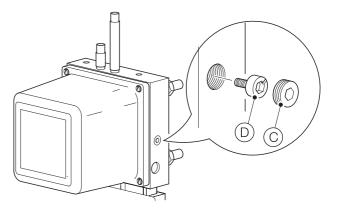
Fig. 7.1 Cleaning / Replacing the orifices
