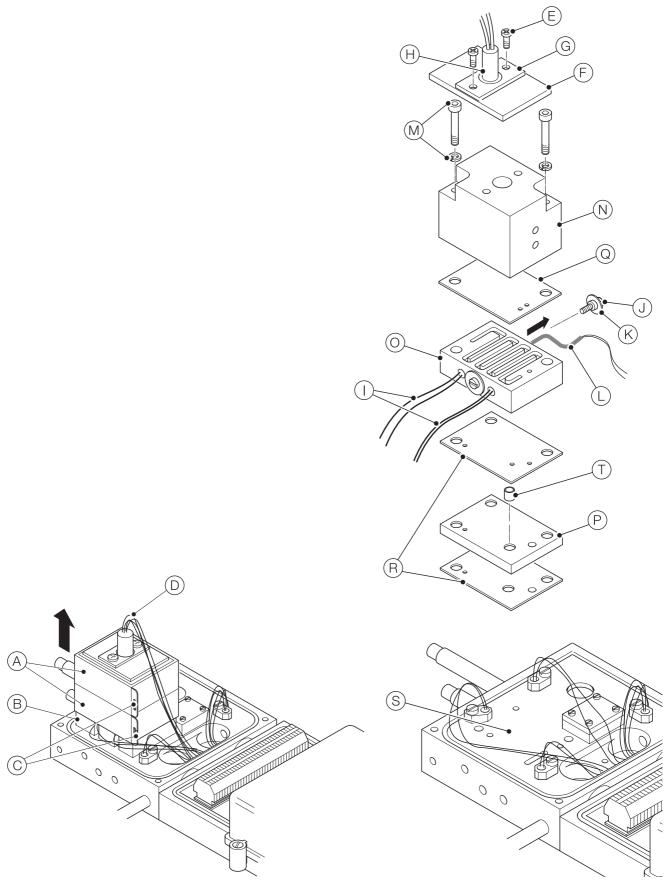
Fig. 8.4 Replacing sensor assembly gaskets
