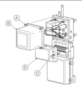
Fig. 8.2 Removing the sensor covers
