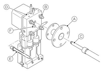
Fig. 8.1 Removing the probe, exhaust filter, adaptor flange from the sensor
