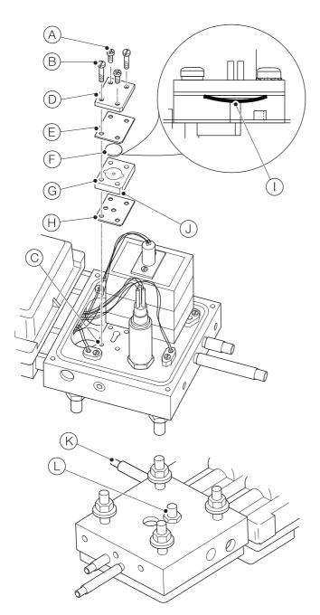
Fig. 8.7 Replacing sensor assembly flow disk
