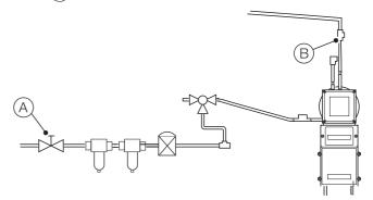
Fig. 5.1 Shutting down instrument air and test gas supplies
