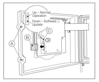
**Caution.** At this point in the procedure, DO NOT restart the analyzer with an SD card in the SD card slot.
