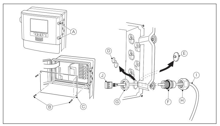
Fig. 4.9 Accessing and Making Electrical Connections
