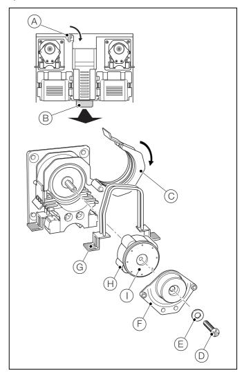
Fig. 8.1 Pump Tubing and Capstan Replacement
