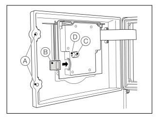
Fig. 9.2 SD Card Removal
