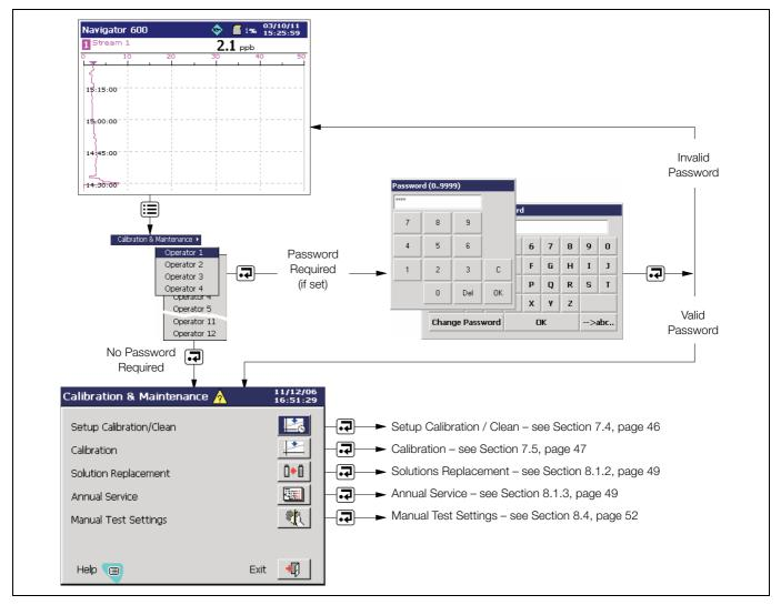
Fig. 7.1 Calibration & Maintenance Overview
