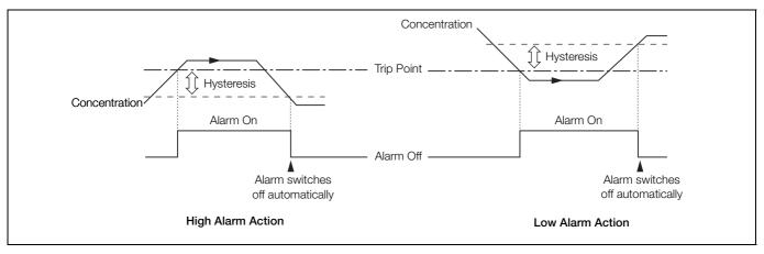
Fig. 5.3 High / Low Process Alarms
