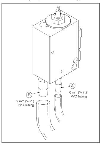
Fig. 4.12 Connecting the Sample Inlet and Drain Line(s)
