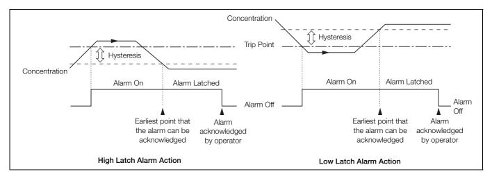
Fig. 5.4 High / Low Latch Alarms
