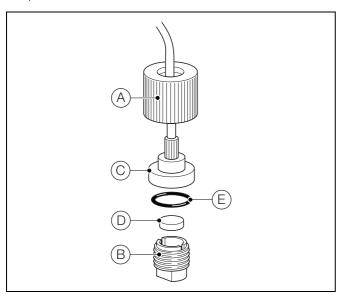
Fig. 8.2 Sample Filter Replacement
