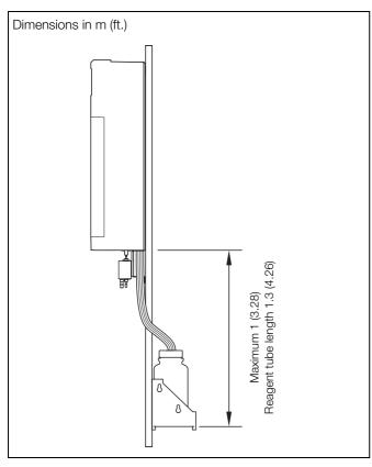
Fig. 4.2 Reagent Bottles Mounted Behind the Mounting Plate or Wall
