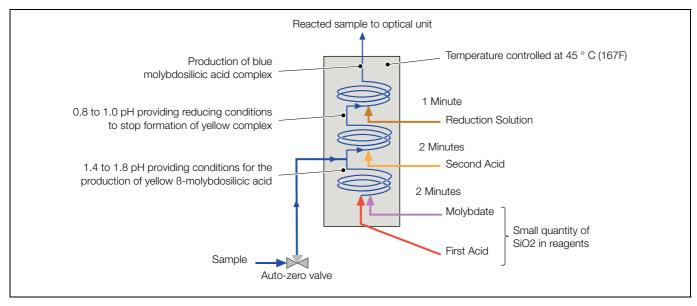
Fig. 7.3 Chemical Schematic During a Zero
