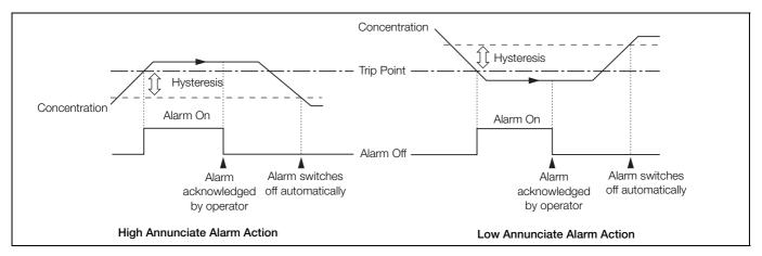
Fig. 5.5 High / Low Annunciate Alarms
