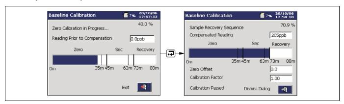
Fig. 7.2 Calibration Progress
