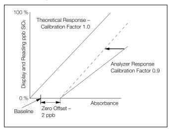
Fig. 7.5 Secondary Calibration
