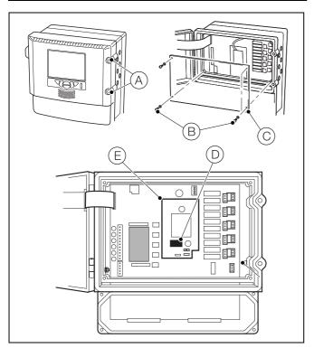
Fig. 8.4 Replacing the DC Fuse
