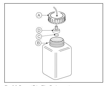
Fig. 8.3 Reagent Tube Filter Replacement
