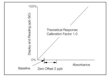
Fig. 7.4 Zero Calibration
