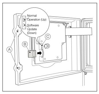
Fig. F.1 SD Card Removal
