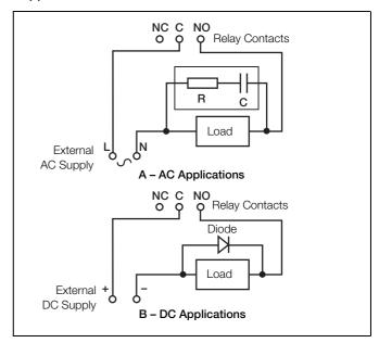
Fig. 4.11 Relay Contact Protection
