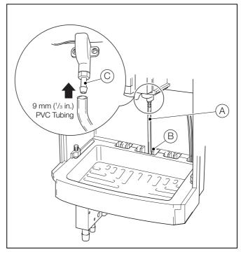
Fig. 4.13 Connecting the Contaminated Drain Tube
