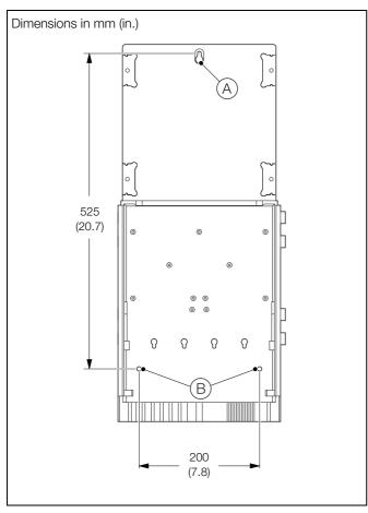
Fig. 4.6 Mounting the Analyzer
