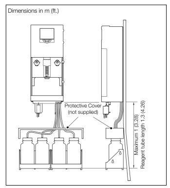
Fig. 4.4 Reagent Bottles Mounted Directly Below the Analyzer
