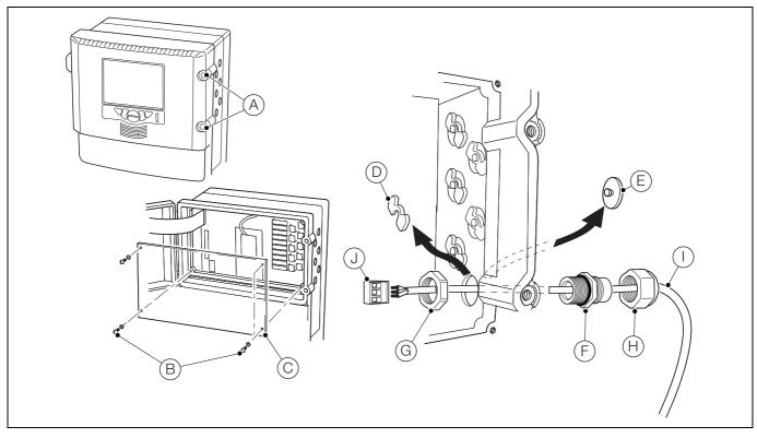
Fig. 4.9 Accessing and Making Electrical Connections
