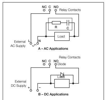
Fig. 4.11 Relay Contact Protection
