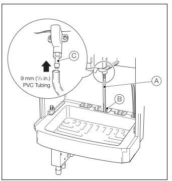
Fig. 4.13 Connecting the Contaminated Drain Tube
