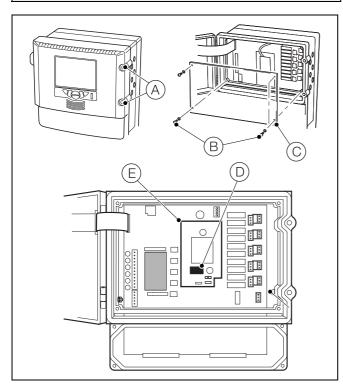
Fig. 8.4 Replacing the DC Fuse
