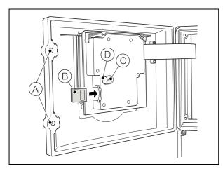
Fig. 9.2 SD Card Removal
