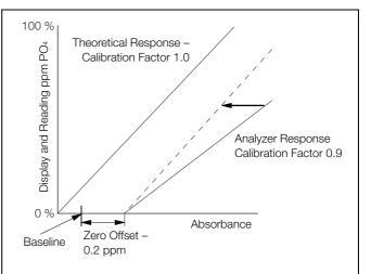
Fig. 7.4 Secondary Calibration
