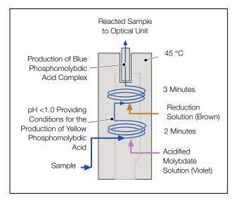
Fig. 3.1 Chemical Schematic
