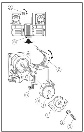
Fig. 8.1 Pump Tubing and Capstan Replacement
