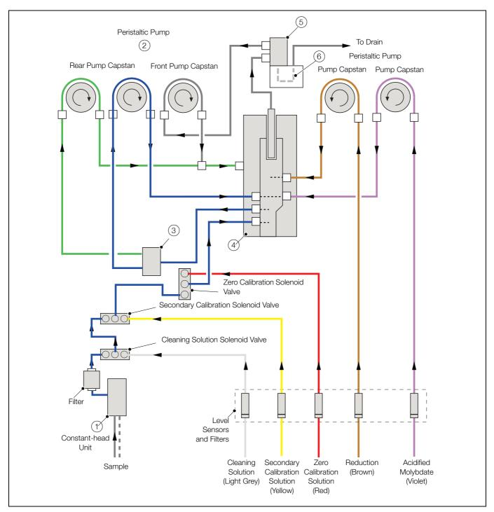
Fig. 3.2 Flow Schematic
