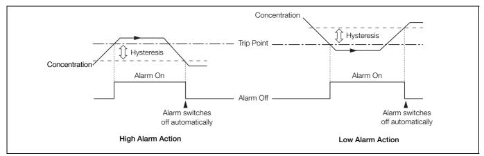
Fig. 5.3 High / Low Process Alarms
