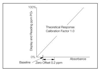
Fig. 7.3 Zero Calibration
