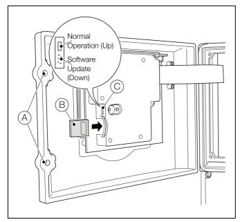
Fig. F.1 SD Card Removal
