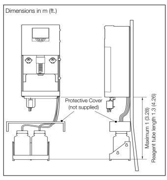
Fig. 4.4 Reagent Bottles Mounted Directly Below the Analyzer
