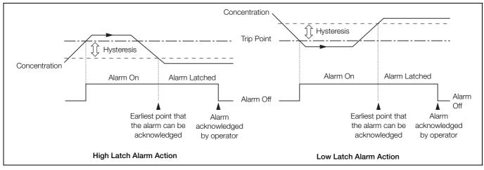
Fig. 5.4 High / Low Latch Alarms
