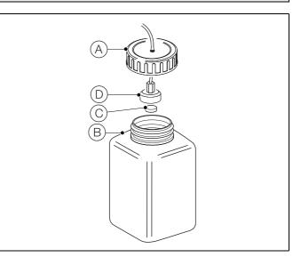
Fig. 8.3 Reagent Tube Filter Replacement
