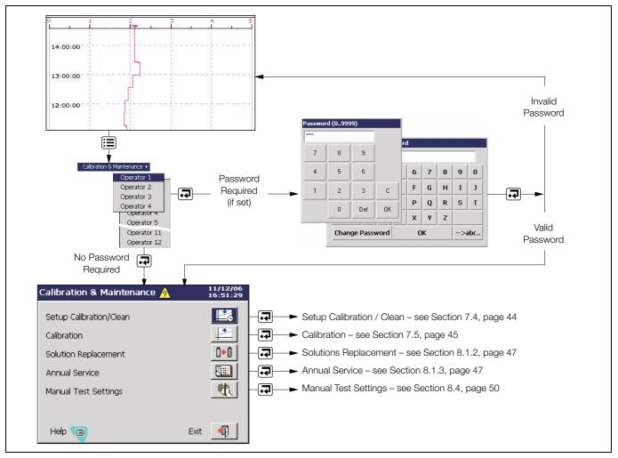
Fig. 7.1 Calibration & Maintenance Overview
