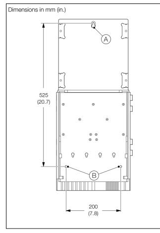
Fig. 4.6 Mounting the Analyzer
