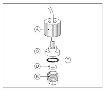
Fig. 8.2 Sample Filter Replacement
