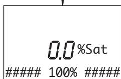
The center display line shows, in the units selected in the **CONFIG. SENSORS** page (Section 5.3), the value to which the instrument's reading will be set following a successful span calibration. If either automatic barometric or altitude correction were selected, the displayed value includes the correction.
