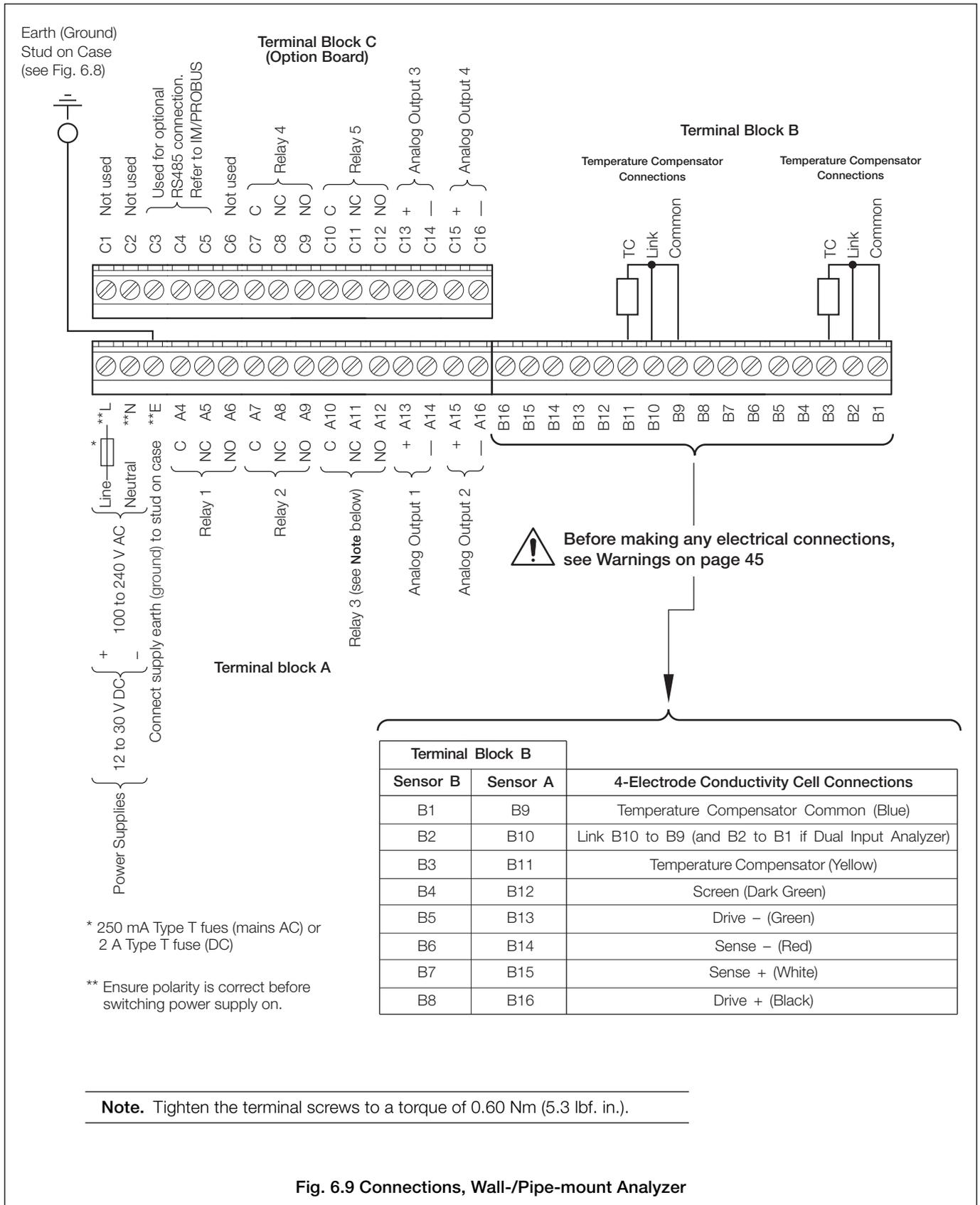
Fig. 6.9 Connections, Wall-/Pipe-mount Analyzer
