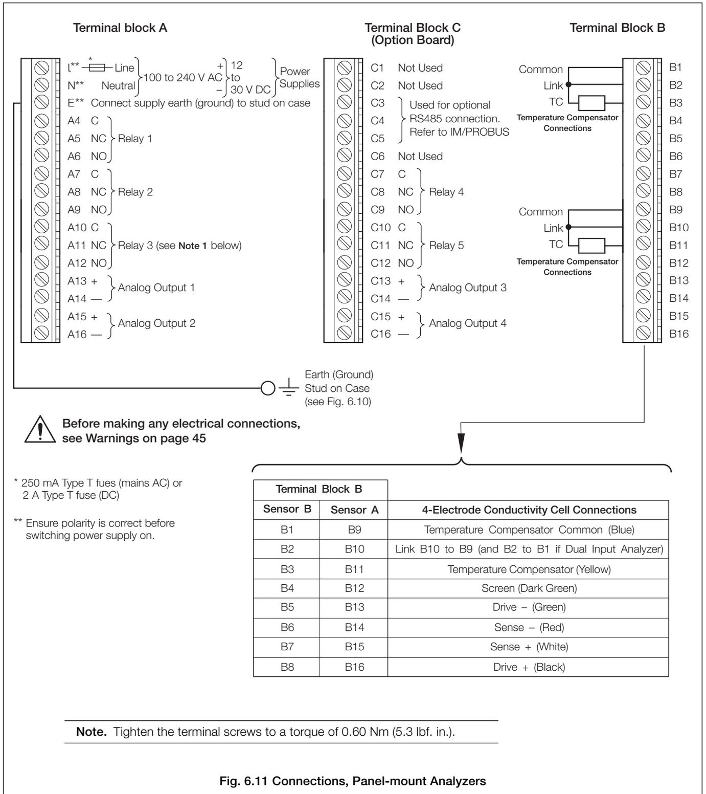
Fig. 6.11 Connections, Panel-mount Analyzers
