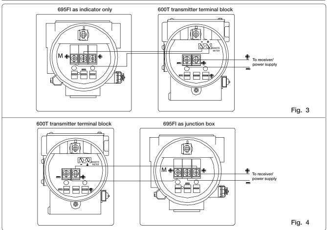
If the terminal block of the transmitter is the latest version with three terminals, the connection is to be realized as explained in pictures 3a and 4a.
