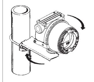
Fig. 1 - Field indicator installation
