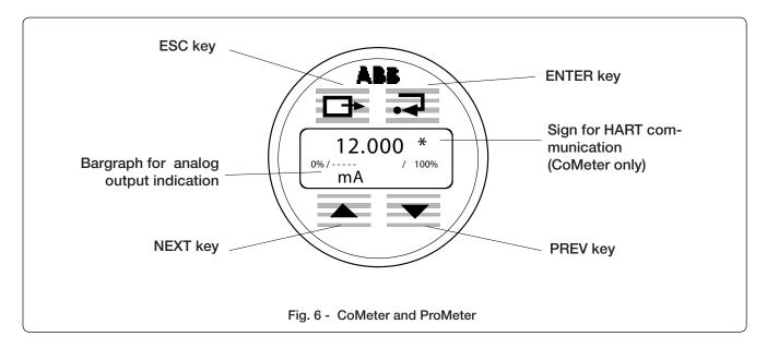
The normal operating condition for CoMeter and ProMeter is to display the analog output signal of the transmitter, expressed in milliAmpere (this is the default setting), or in percentage or in engineering unit, with all the units available as for the HART Communication Protocol.
