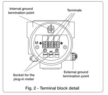
The field indicator can be connected in accordance with the following two configurations:
