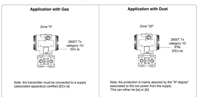
b) Certificate ATEX II 1/2 GD T50°C, EEx ia IIC T6 (-40°C ≤ Ta ≤+40°C) respectively, GD T95°C, EEx ia IIC T4 (-40°C ≤ Ta ≤+85°C)
