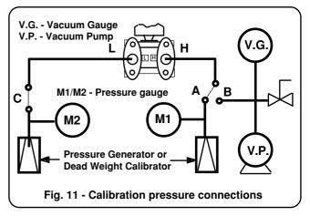
Note that calibration accuracy is strictly related to the accuracy of the test equipment: the use of a dead weight tester is highly recommended.
