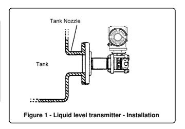
The liquid level transmitter has been designed to connect to a flanged tank nozzle, or similar ANSI (DIN) fitting. Standard connections for 2/3-inch Class 150/300/600 flanges, and equivalent DIN, are available.
