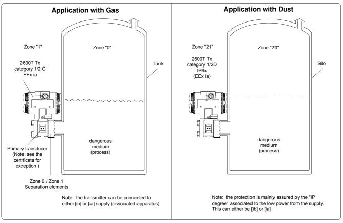
c) Certificate ATEX II 1/2 G Ex d IIC T4+T6 and or ATEX II 1/2 D Ex tD A21 IP67 T85°C (-50°C ≤ Ta ≤+75°C)
