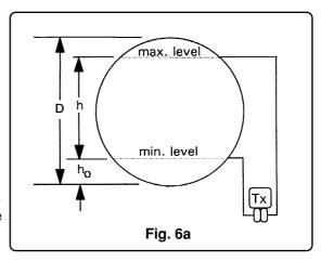
If it is required the partial volume starting from  $\hbar$  (i.e. the volume at  $\hbar = 0$ ) then the Accoefficient should be equal to the polynomium solved for  $\hbar$ 0 with negative sign: for example for  $\hbar$ 0 = 20%
