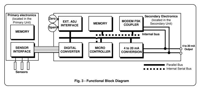
With secondary electronics analog+HART, it is to be consider that different communication protocols exist for configuration and maintenance operations. Here follows a brief description on the matter; please refer to appropriate technical specification. It is also possible to read other transmitter data and diagnostic for additional deeper explanations on the communication aspects.
