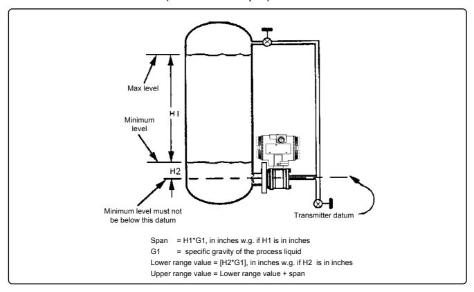
Application n° 3 : Liquid Level - Closed Tank Using a Flange-Mounted Transmitter and a Wet Leg (With Condensable Vapors)
