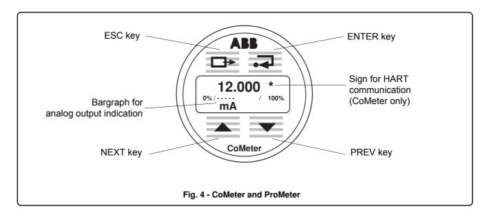
The normal operating condition for the CoMeter is to display the analog output signal of the transmitter, expressed in milliAmpere (this is the default setting), or in percentage or in engineering unit, with all the units available as for the HART Communication Protocol.
