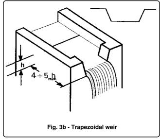
Using this function, the output (in % of the span) is proportional to the square root of the third power of the input signalri % of the calibrated span: the instrument, e.g., gives an output proportional to the rate of flow calculated using the above mentioned formulas.
