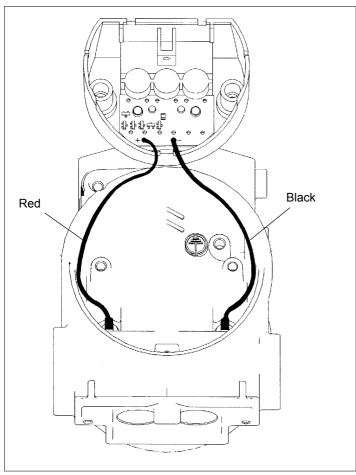
Fig. 2a Connection for terminal block and housing.
