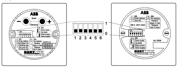
Switch 1 and 2 are used for Snap Calibration, Zero and Span Raise/Lower and also for Damping step.
