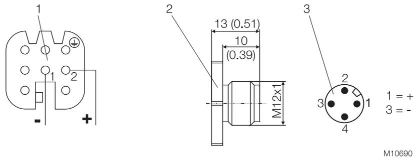
**Fig. 9: Pin assignment**
