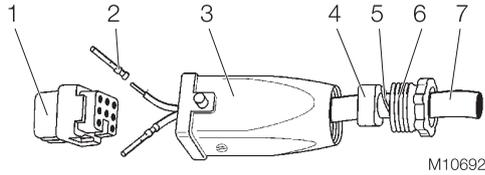
**Fig. 10: Assembling the socket connector**
