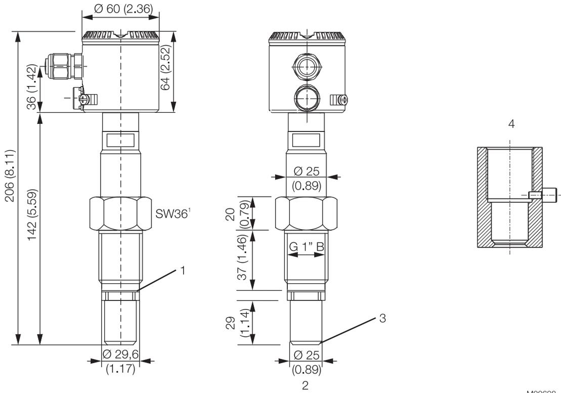
Fig. 27: Dimensions - With ball valve connection
