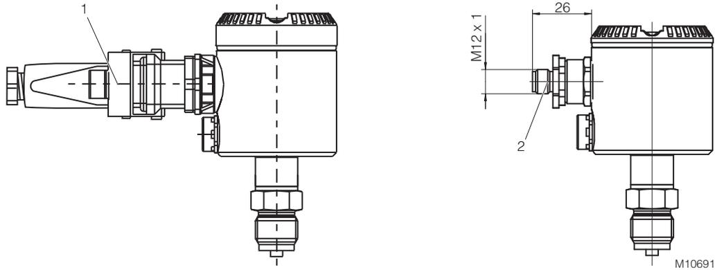
**Fig. 8: Connection via plug connection**
