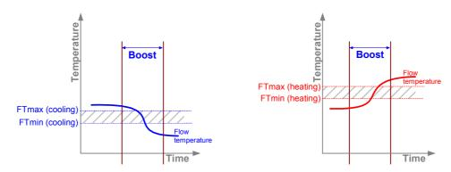
In Heating Optimisation, the flow temperature must be below the minimum temperature in the range, (i.e. below the value of FTmin) at the start, and must rise past the maximum temperature (FTmax) during the boost period.
