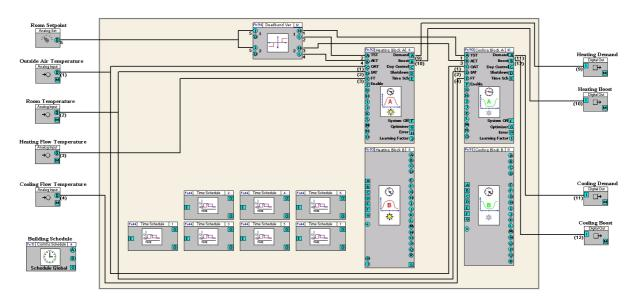
The inputs on Optimiser block A (in both Heating and Cooling) must be connected as shown above. The outputs can then be connected to the Demand and Boost points as shown.
