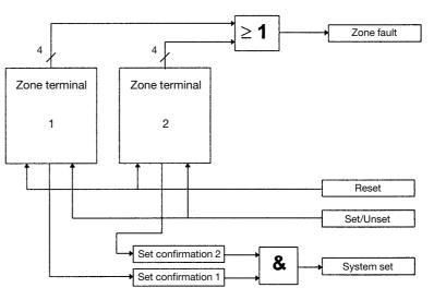
The telegram 'System set' is produced by a logical AND connection of all 'Set confirmations'.
