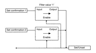
In order to activate the system, a telegram 'set/unset' with the value '1' is sent as usual. The value '1' also allows the filter gates to be enabled which have been programmed so that they only allow the value '0' to pass through. Once the set telegram has been received, the zone terminals report back either with the value '1' (set) or '0' (unset).
