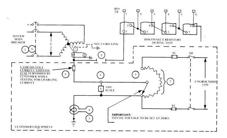
Figure 3. Testing Schematic
