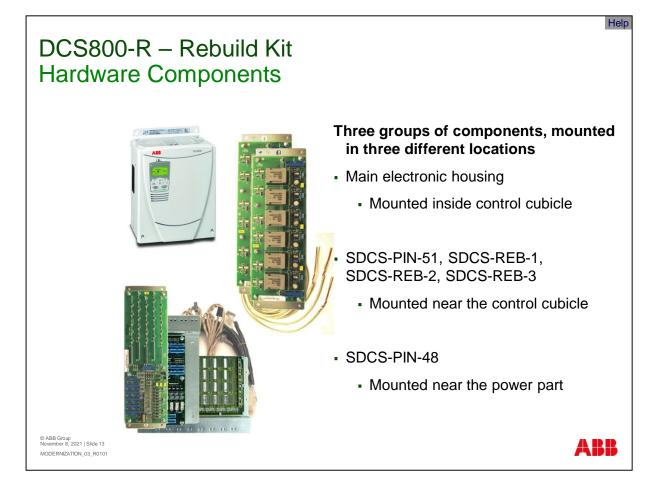
Let us have a closer look at the hardware components of the DCS800 rebuild kit. We can divide the components into three large groups, because the mounting location is different.
