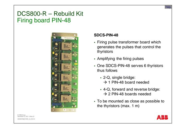
The PIN-48 is the firing pulse transformer board which generates the pulses that control the thyristors. In principle, it amplifies the firing pulses. One PIN-48 board serves 6 thyristors.
