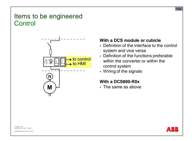
Another important issue for engineering is the control section. Some drives are controlled by hard wire signals and other ones can have a fieldbus connection.
