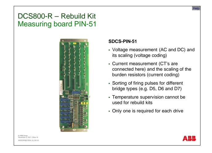
The PIN-51 board is very important for rebuild kit engineering.
