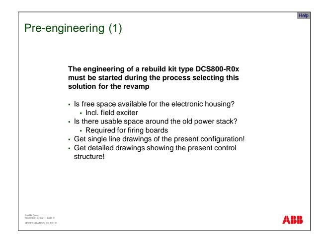
Pre-engineering is the step which typically starts the process of selecting the DCS800-R rebuild kit as a solution.
