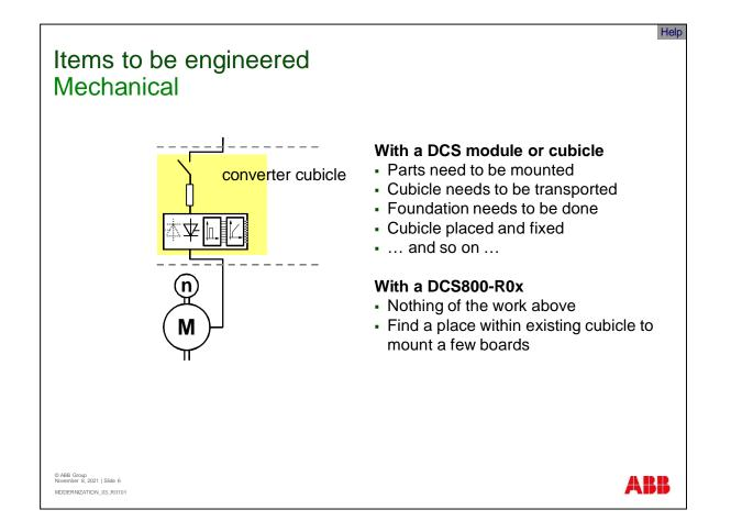
Typically, the first item to be engineered are the mechanics. Only if the mechanics are clearly defined, electrical points be considered.
