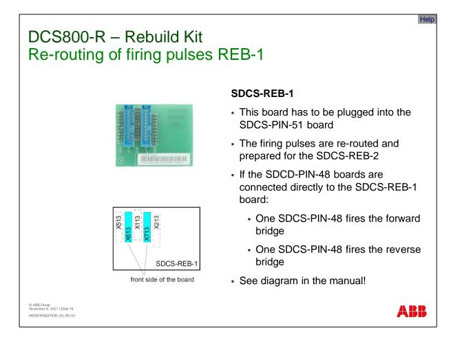
Re-routing of firing pulses is possible with the REB-1 board.
