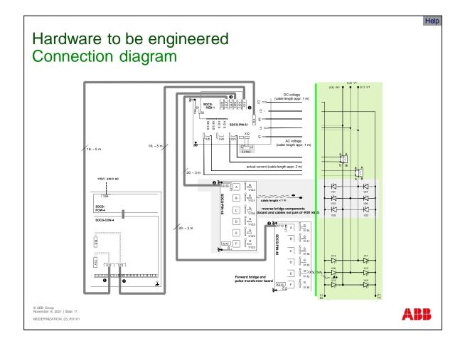
The picture shows the principle connection diagram for the DCS800 rebuild kit. On the right hand side of the green line is the power part, which will be reused. The power part consists of at least a single bridge used for 2-quadrant mode. In historic circuits, it is possible to have thyristors in parallel because in former times the power of the thyristor was limited.
