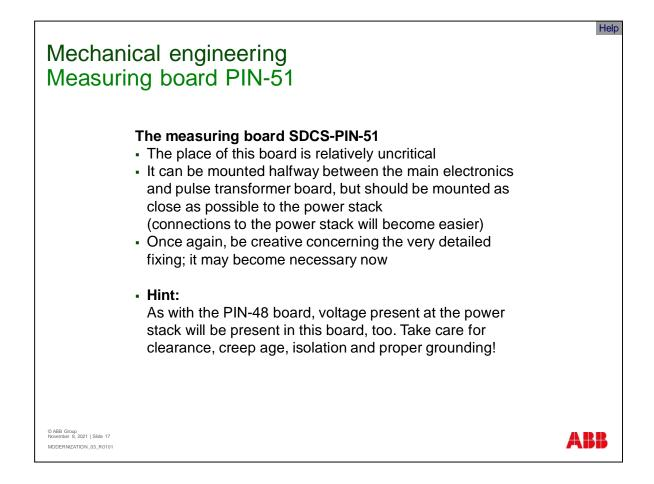
The measuring board PIN-51 must be engineered. Therefore some points need to be discussed here:
