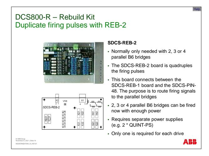
The REB-2 board is used to duplicate firing pulses.
