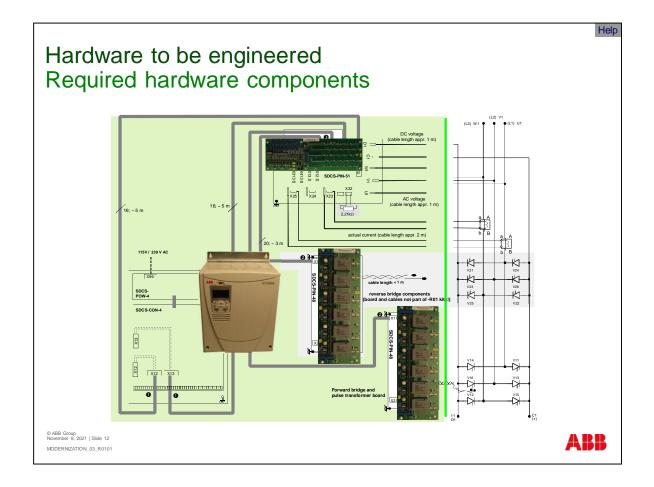
The required hardware components for the rebuild kit are shown in the picture. The main part in the electronic housing, is connected to some other electronic boards. Only the electronic housing, the electronic boards and the cables are contents of the rebuild kit. Thyristors, current transformers and main switches should be reused or modernized, if necessary.
