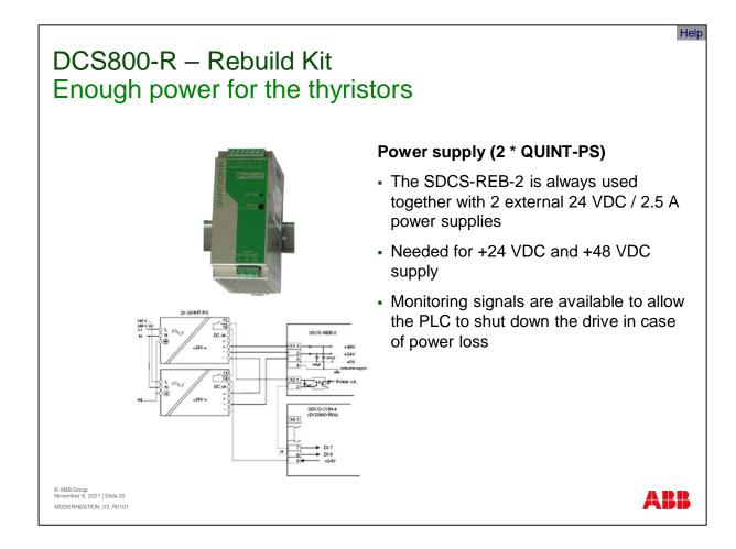
The connection diagram shows how to connect the two power supplies. Then 24 volts and 48 volts are available at the REB-2 board.
