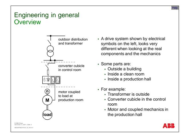
A drive system, shown by electrical symbols on the left, looks very different when looking at the real components and mechanics.
