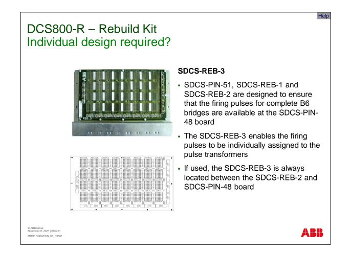
Sometimes a customized design is necessary. The REB-3 board provides a free design area for the PIN-48 board. Then the REB-3 board enables the firing pulses to be individually assigned to the pulse transformers. If used, the REB-3 board is always located between the REB-2 and the PIN-48 board.
