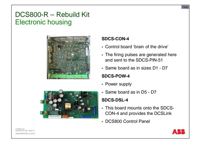
The electronic housing consists of at least the following components.
