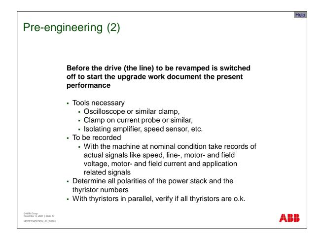
Before the drive or production line to be revamped is switched-off to start the upgrade work, it is helpful to document the current performance.
