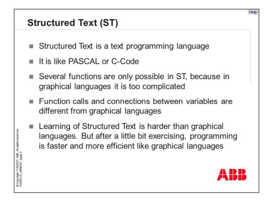
"Structured Text" is a text-based programming language in CoDeSys. It is similar to PASCAL or C-Code. Several functions are only possible in "Structured Text" because in graphical languages it is too complex. Function calls and connections between variables are different from graphical languages. Learning of "Structured Text" is harder than graphical languages. But after a little bit exercising, programming is faster and more efficient like graphical languages.
