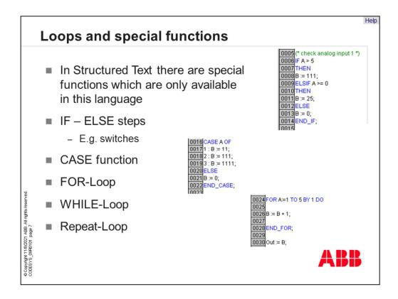
Next special function are the loops. In "Structured Text" it is easy to define loops directly like in C-Code or Pascal. Another important function is the "IF-ELSE-Construction". With this it's easy to program switches. Also important is the "CASE-Command". You can use it for selections from a volume.
