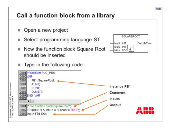
In graphical languages a call of a function block is easy to do when you put in function blocks. In a text language the function block isn't visible at all. You see only a line with variables and allocations. But with "Structured Text" you can do the same things and more as with graphical languages.
