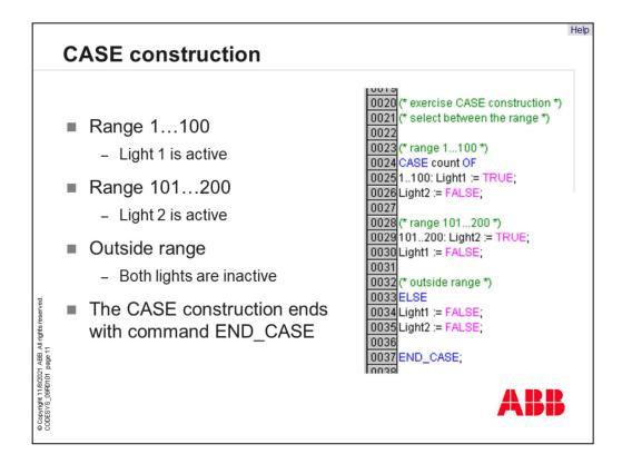
The "CASE-Construction" looks like the picture on the right side. We have 1 variable, here "count", and the several steps with the defined range. It ends with the command "END\_CASE".
