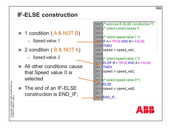
Let's have a look to the "IF-ELSE-Construction". Each "IF-Condition" has a boolean expression to select if the expression is fulfilled. If it's fulfilled the command will be executed. Otherwise, the next step is checked. The whole construction ends with the command "END\_IF". So, you can define a stairs with several steps which can be executed or not.
