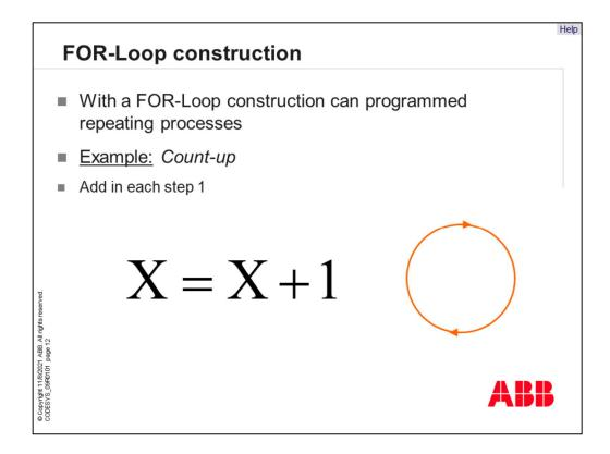
Another important function is the "FOR-Loop-Construction". It have the functionality like a counter because the loop will be executed as long as the condition is fulfilled. An example is an upward counter. The user defined the starting point and the end point. Later the loop runs from the starting point to the end and increase the counter value with each cycle.
