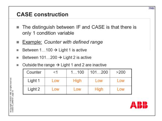
Now we change to the "CASE-Construction". The distinguish between "IF" and "CASE" is that there is only 1 condition variable. This variable has more than 2 conditions and the "CASE-Construction" checks the actual state of the variable. Then it comes a decision!
