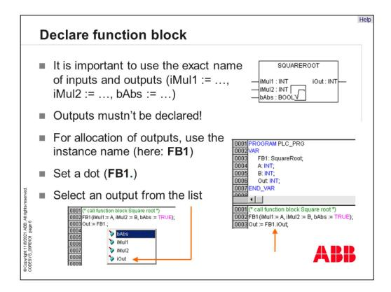
Inside the brackets you can see the several inputs. After the equal sign you can set the connection variable. It is important to use the exact name of inputs and outputs, otherwise you get error messages. Outputs mustn't be declared. For allocation of outputs, use the instance name, here FB1.
