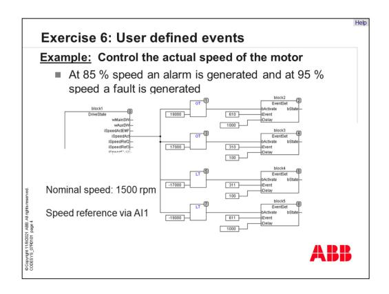
Let's do a little exercise. We would like to control the actual speed of a motor. At 85% of nominal motor speed there should be generated an alarm and with 95% a fault. The application should have the functionality for both motor directions.
