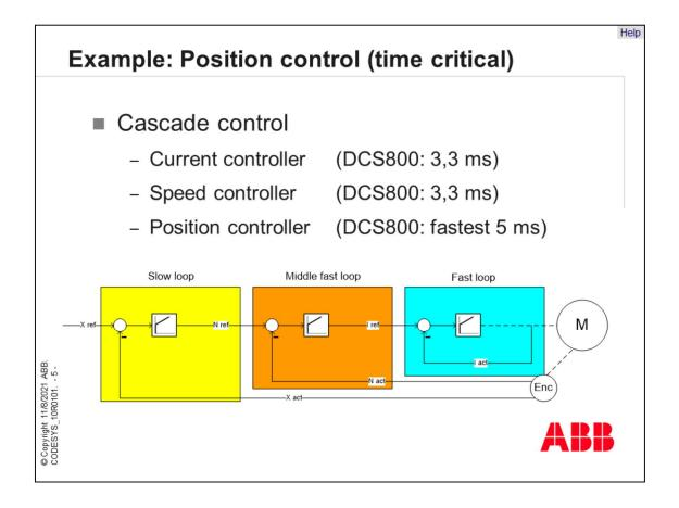
An example of a time critical application is a position control. To generate this application the current and speed controller are used from the standard firmware. The execution time of these control loops is 3,3 milliseconds. The position controller has to work in the fastest task cycle in CoDeSys with 5 milliseconds. Slower execution cycles would cause to problems for the entire control performance.
