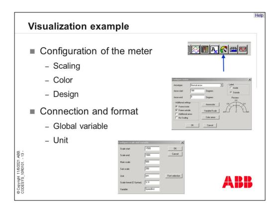
All devices used in the visualization window must be configured to show the correct values. The first device is the meter which should be used to display the actual speed of the drive. Important settings for the meter are scaling, color and design.
