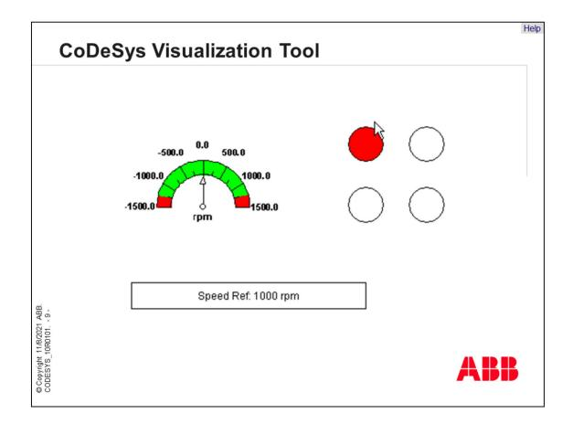
CoDeSys includes a visualization tool which can be used to connect global variables of the program. The visualization tool offers several buttons and fields to get status signals or to set reference values.
