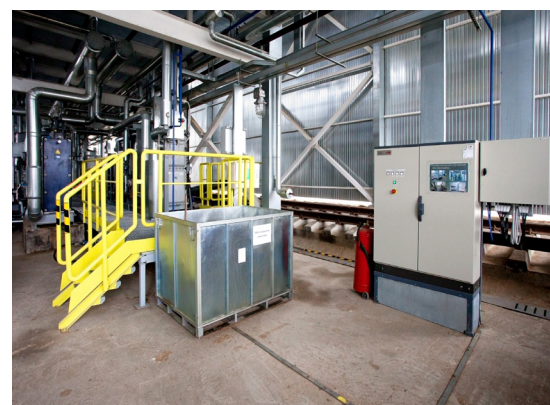
Lubcel™ interface in wagon/truck bulk material loading station
