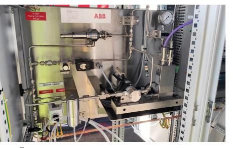
The In-Line Colouring System developed by ABB enables the dyeing of lubricants directly during bulk loading operation without any prior dilution of colorants. It guarantees an on-spec coloured product, while reducing energy and space requirements.
