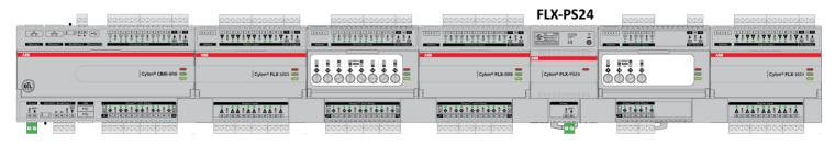
FLX-PS24 facilitates remote connection of FLX I/O modules to CBXi or CBX to a maximum overall length of 1200 m (3280 ft). Each FLX-PS24 can power a bus segment of up to 30 m (100 ft):
