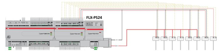
The number of FLX I/O modules that can be powered by a FLX-PS24 depends on the model and loading of the individual FLX I/O modules. Any combination where the total full-load power is less than 20 W can be used. The Power Consumption table below shows the power load of each FLX I/O module:
