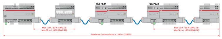
FLX-PS24 can provide 20 V DC DIN rail-mounted power supply for external field devices using the FLX-RMC:
