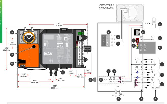
**Note:** In the CBT12iVAV, terminals 3, 18 and 33 are connected internally.
