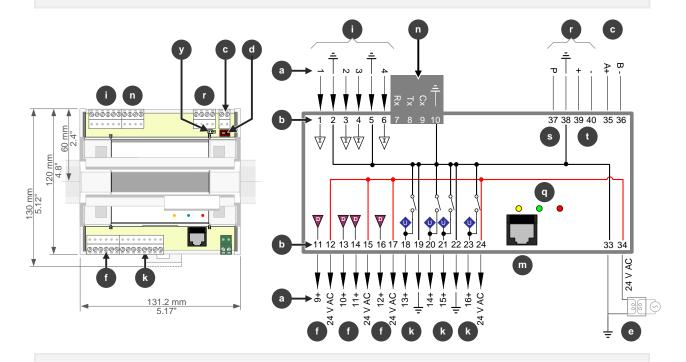
**Note**: In the CBT12, terminals 12, 15, 17, 24, and 34 are connected internally. When a controller is powered, 24 V AC is available for low current devices at terminals 12, 15, 17, and 24. The total combined current must be less than 0.9 A.
